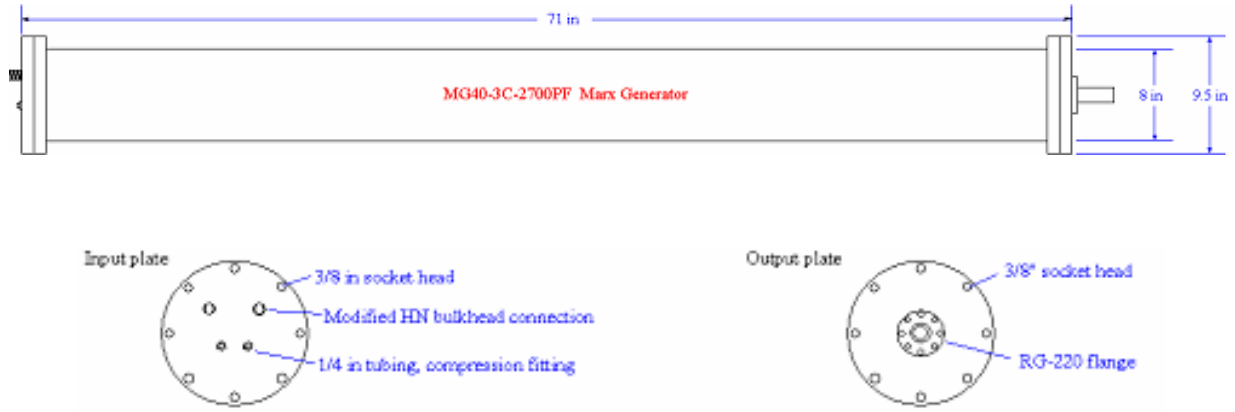
Figure 5. A dimensional view of the APELC MV Marx generator
