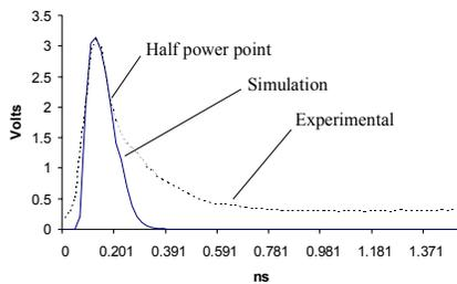
Figure 6. Experimental and simulation results for the first material. Recombination time of 30 ps.
