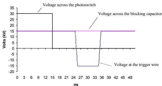
Figure 8. Simulation results for triggering a field distortion gap with a traditional photoswitch circuit.
