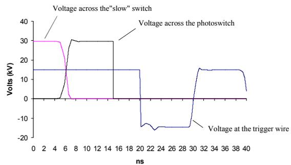
Figure 12. Simulation results of the waveless-charge photoswitch trigger.
