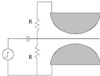
Figure 3. The field distortion spark gap with a blocking capacitor.
