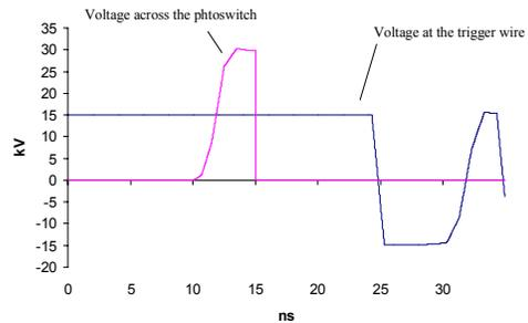
Figure 10. Simulation results of the transient-charge photoswitch trigger.
