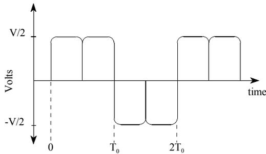
Figure 3. Alternate pair charging output waveform.
