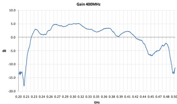
**Figure 11.** Gain Measurement of the Helical Antenna
