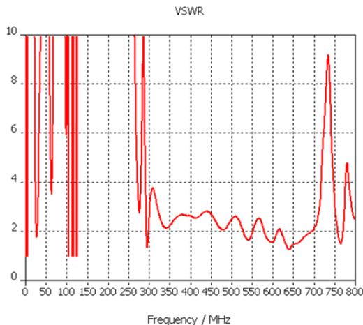
**Figure 6.** Simulated VSWR for the 400 MHz Helical Antenna
