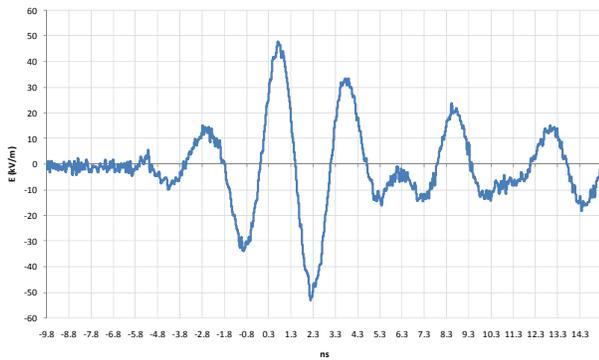
**Figure 14.** Radiated Signal From the Helical Antenna
