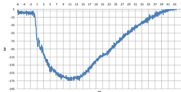
**Figure 13.** Driving Voltage Pulse From the Marx Generator
