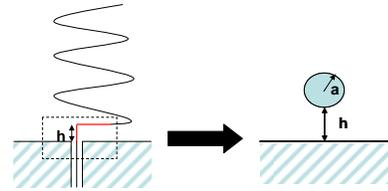
**Figure 4.** Illustration of the Rod-Over-a-Ground Plane with Definitions
