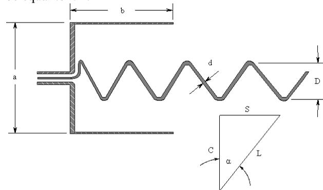
**Figure 5.** Cupped Ground Helical Antenna Defined by Kraus
