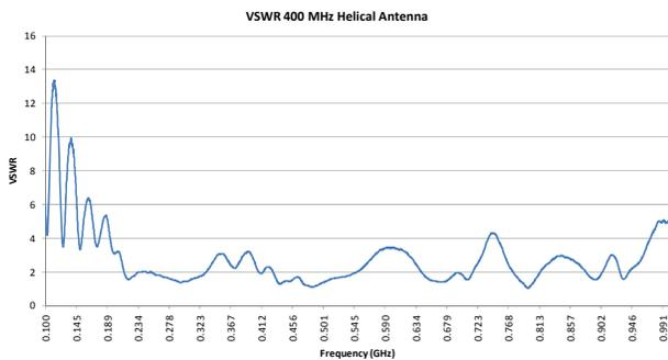
**Figure 10.** Measured VSWR for the 400 MHz Helical Antenna
