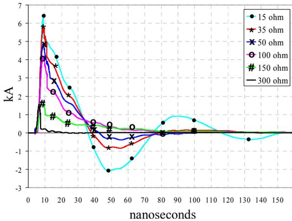
**Figure 6.** Output waveforms with a 30 kV charge.
