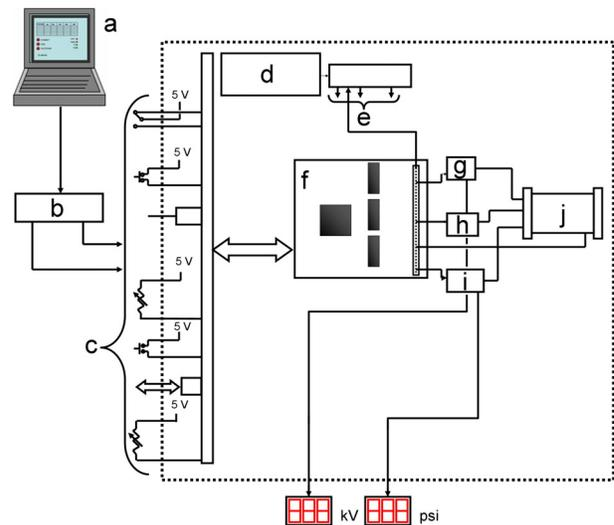
**Figure 2.** Controller block diagram. (a), *LabView* P.C. (b), RS-232 to Fiber (c), local/remote controls (d), 30v battery-pack (e), 5, 12, 28 Volt outputs (f), HCS12 Microcontroller (g), H.V. Power-supply (h), Electronic Pressure-regulator (i), Trigger-generator (j), Marx Generator
