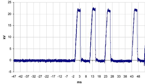
**Figure 7.** Charging waveform for 100 Hz operation.
